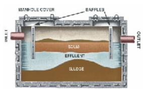
inert solid materials and the by-products of bacterial digestion accumulate.
